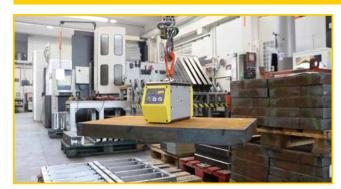
Battery-powered lifters for lifting and handling ferrous loads of various shapes and sizes.
