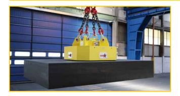
Electro permanent lifters for the handling of slabs and forged blocks with an increased air-gap.
