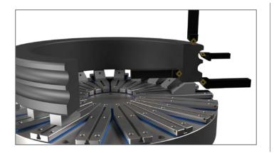
Thanks to the absence of bulky components conventional clamping systems are composed of, this magnetic system allows wide access to the machinable areas of the work-piece.
