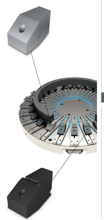
The use of pole extensions increases the distance between the chuck and the work-piece by maximising access to the free surfaces of the work-piece for through-hole drilling and complete longitudinal turning.
