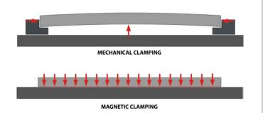
Unlike brackets and vices, which only act on the workpiece with concentrated forces, the magnetic chuck clamps evenly its entire contact surface.
